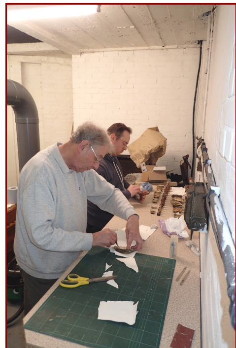
Above: John Smallwood and Richard Hills releathering wooden flue pipe tuning stoppers
